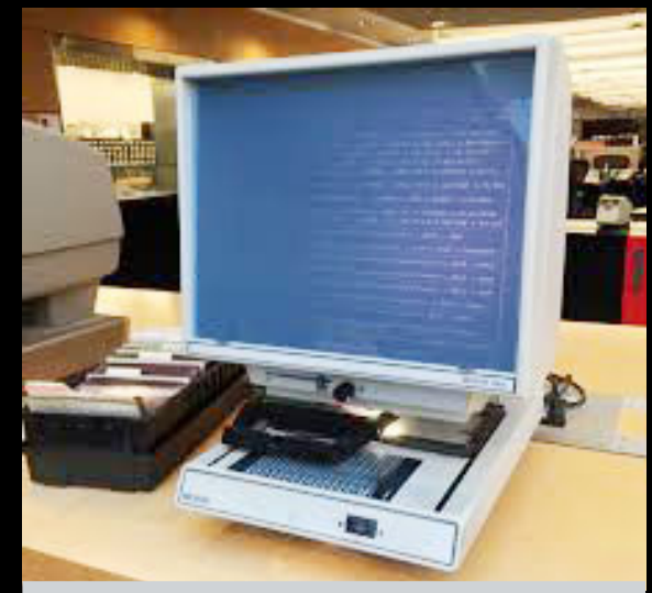
A Rigler Deutsch Index microfiche reader which was used to magnify and display microphotographs of documents stored on sheets of film. (Image courtesy of commons.wikimedia.org)
